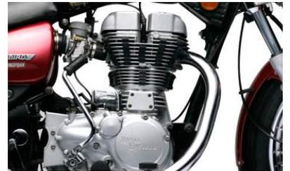
Unit Construction Engine
