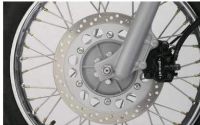
Brake (280MM Disc - Front Brake
